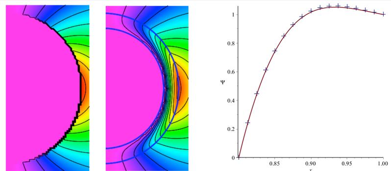
**Left:** Numerical solution initial condition. **Right:** The system relaxes to a Hall equilibrium where the toroidal field is confined in the closed tori.
